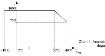
Chart 1. Acceptable output current from the PSU depending on ambient temperature.
